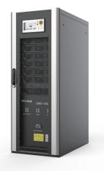
Model: **CMS-150/25** Max. Capacity of system: **150KVA** Configuration: **6 slots** Power module model: **CM25** Power module capacity: **25KVA** Dimension: **600\*1000\*1600**(W\*D\*H)mm, standard 19″ cabinet
